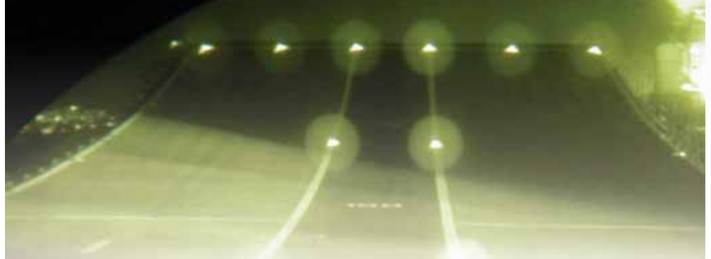
Looking at Ark Royal's ramp with Gen III, Omni IV goggles with the deck end/centreline light on. Stray light on the deck comes from Portsmouth harbour, as the ship is in dock in this picture.
